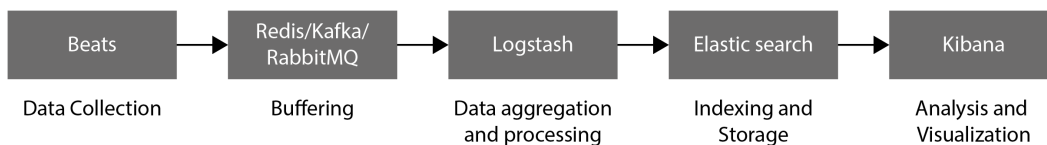
Figure 7.2 – High-level architecture of the ELK stack
